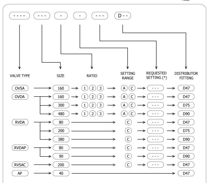
(\*) If not specified, the valve will be supplied with the standard setting. Refer to the valves datasheets for the standard setting value.
