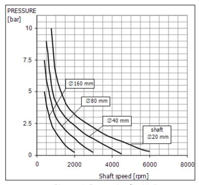
Diagram 1: Pressure Loading Limits
