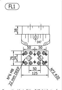
Connection block, fitting D47 distributor, for motor MR 125/160/190/200/250/300/330
