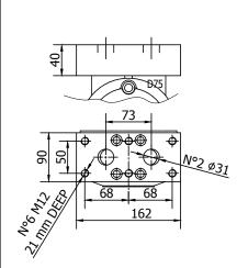
Connection block, fitting D75 distributor, for motor MR 1100/1400/1600/1800/2100
