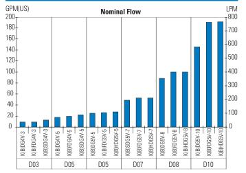
Nominal flow rated @ 5 bar delta P, single path except for K(B)SDG4V-3/5 valve rated @ 35 bar delta P, single path
