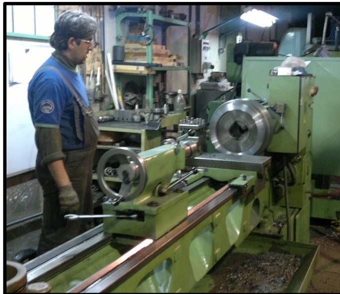
Figure 2 -3) in order to couple variable pump to diesel motor some accessories are required, for making special type bell housing and coupling. These parts are in machining process now
